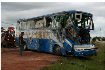
Figure 3-4: Extended Damages on the Right of the Bus
