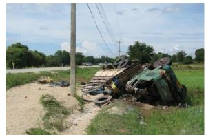
Roadside Embankment (left side) Rest Position Partly on Paddy-field Figure 3-16: Unsafe Roadside Slope-Roadside Embankment
