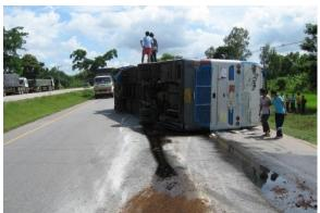
Roll-over of 10-Wheel Truck (0.375) Roll-over of 6-Wheel Bus (0.25) Figure 3-14: Rest Positions of Rolled-over Vehicles
