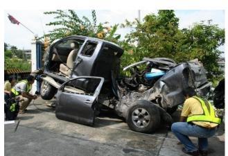
Figure 3-3: Deformed Pickup Bed
