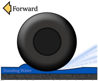
Figure 3-9: A diagram of a hydroplaning tire Source: Wikipedia, 2009
