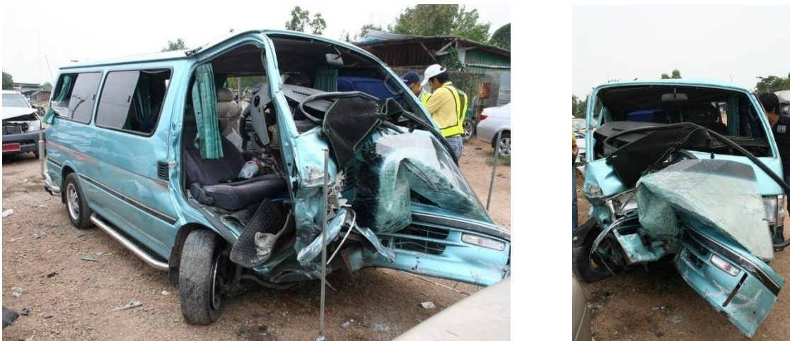
Figure 3-4: Frontal Deformation of the Van
