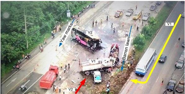
Figure 16 Sequences of the Accident Provided with Evidences (Yaw Marks and Barren Lawn)
