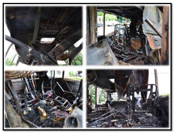
Figure 13 Damages inside the Bus
