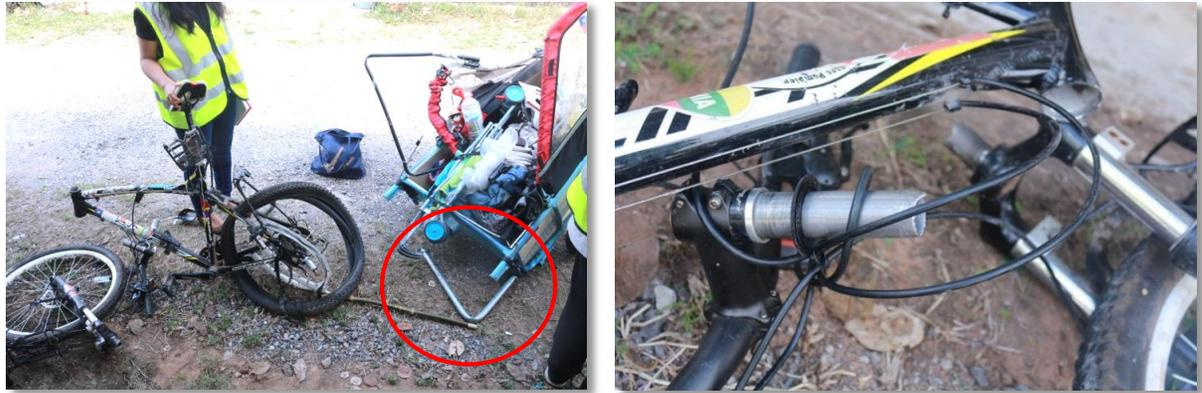
**Figure 17 Damages of V2, (broken connecting rod, frame and handle)**
