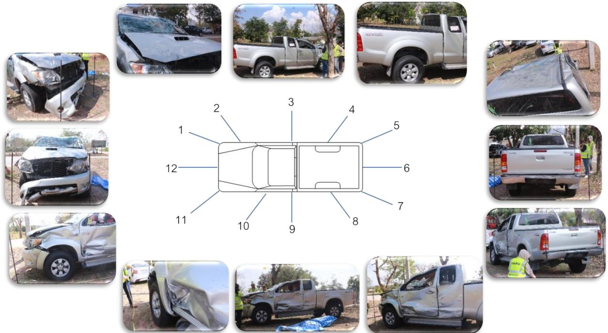
**Figure 13 Damage condition of the pickup from all directions**
