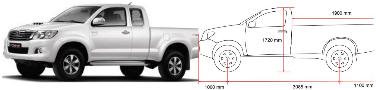
**Figure 7 Original structure of the pickup, dimension of the pickup**
