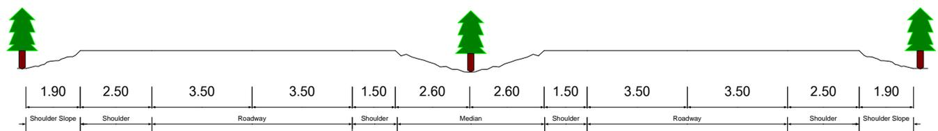
**Figure 21 Typical cross section of Hwy no.2**
