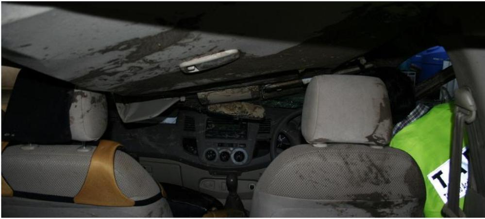
**Figure 3-12: Deformed Roof Interior**
