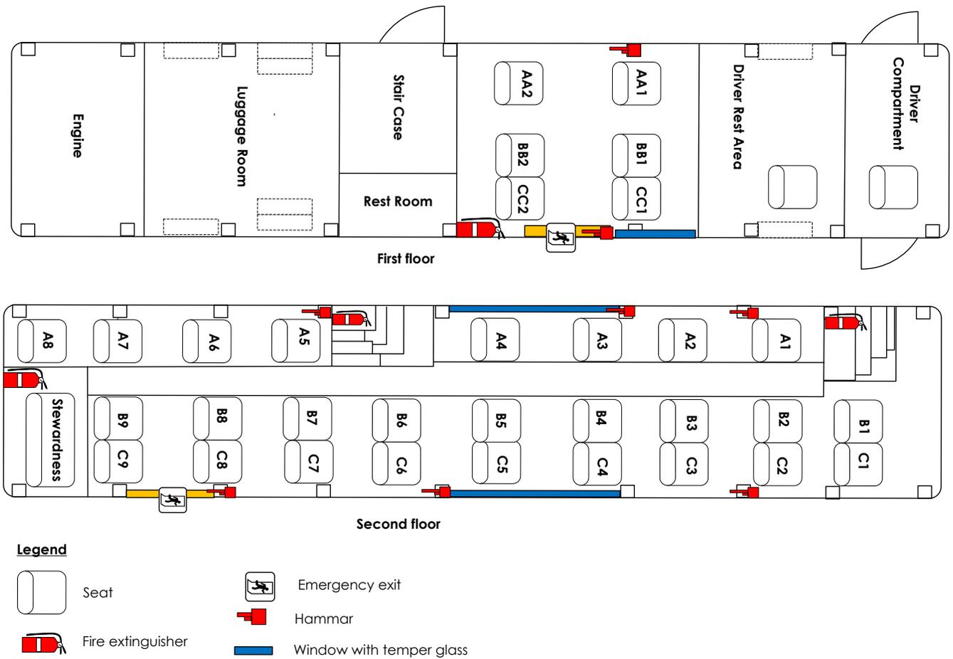
**Figure 6 Seat position and Location of Safety Equipment's**
