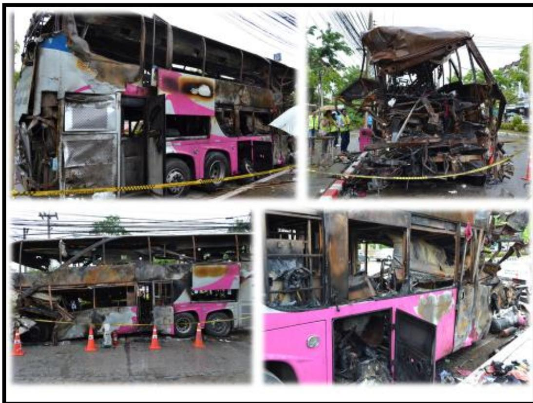
**Figure 12 Damages of the Bus**
